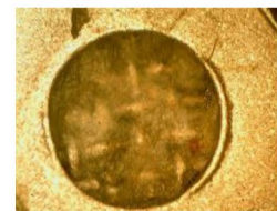
Further magnification shows the biofilm covering the wire mesh reducing spray flow.
