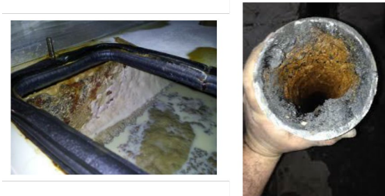
Figure 4 - A biofilm located on top of the die lubricant diluted tank (left); Biofilm build up in a pipe line supply die lubricant to the Die Cast Machines. Notice the that the pipe diameter is almost reduced by 50% (right).
